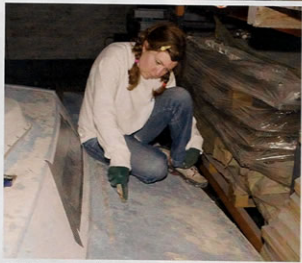
ABOVE and RIGHT Stripping the deck paint using the chemical stripper proved frustratingly slow
