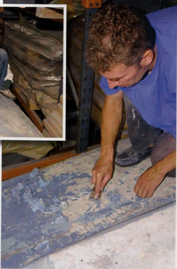
ABOVE and RIGHT Stripping the deck paint using the chemical stripper proved frustratingly slow
